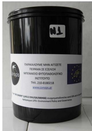
**Figure 7.** Ovitrap with a label
