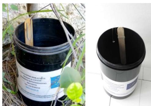
**Figure 1.** Ovitrap components and tool; left: black container and tongue depressor; right: fish descaling knife to scratch the tongue depressor.
