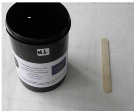
Figure 1. Ovitrap components: black container (left) and tongue depressor (right).
