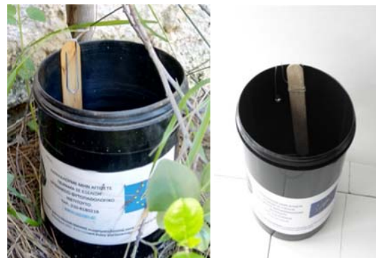
Figure 2. The final set up of the ovitrap ready for placement.
