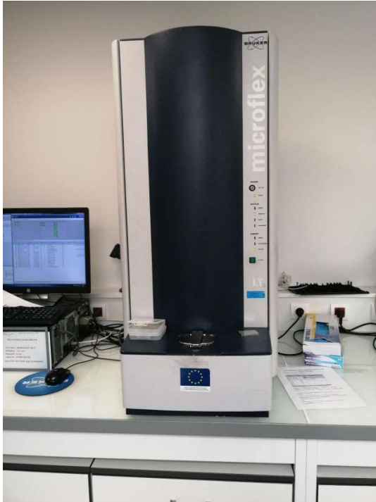
Mass Spectrometer device used for the study Microflex LT MALDI-TOF (Bruker Daltonics, Germany)
