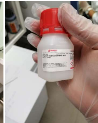
Preparation of the matrix composed of saturated \alpha -cyano-4-hydroxycinnamic acid, 50% acetonitrile and 2.5% trifluoroacetic acid
