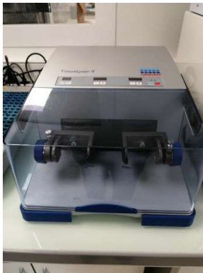
Automatic homogenisation of the samples using acid washed glass beads and TissueLyser II(Qiagen)
